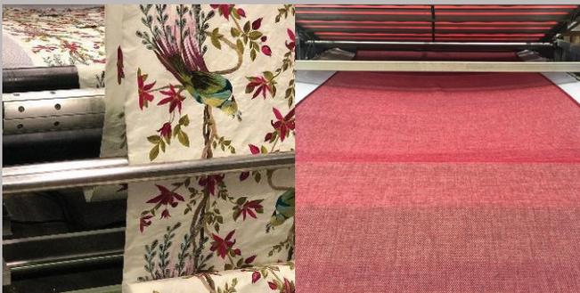
**Spray-on/Air-dried:** Chemical is sprayed onto the textile/fabric until the fabric is completely saturated, thicker fabrics need a heavier coat of fire retardant and will often take double the drying time. Standard textile fabrics usually takes 8-24 hours to dry completely.
